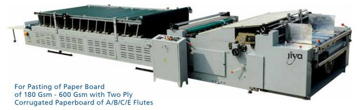
The Laminator Uses Vacuum-Sucking Paper Movement Type For The Bottom Paper & Top Paper Is Fed Manually By Hand For Easy Operation & Maintenance
