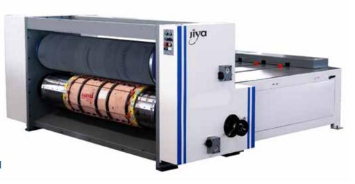
It is equipped with auto recovery device. It can be repaired 4-5 times in normal condition. At the same time, it uses speed difference device without operator intervention, and automatically adjusts the roller speed. Ensure that each batch of carton size is fully consistent.
